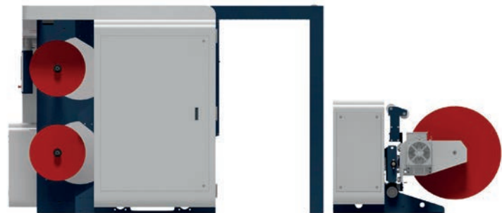
D Overhead web path: rewind on the opposite side of unwind
